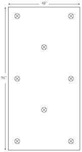
Fasteners should be a minimum of 3" from edge
