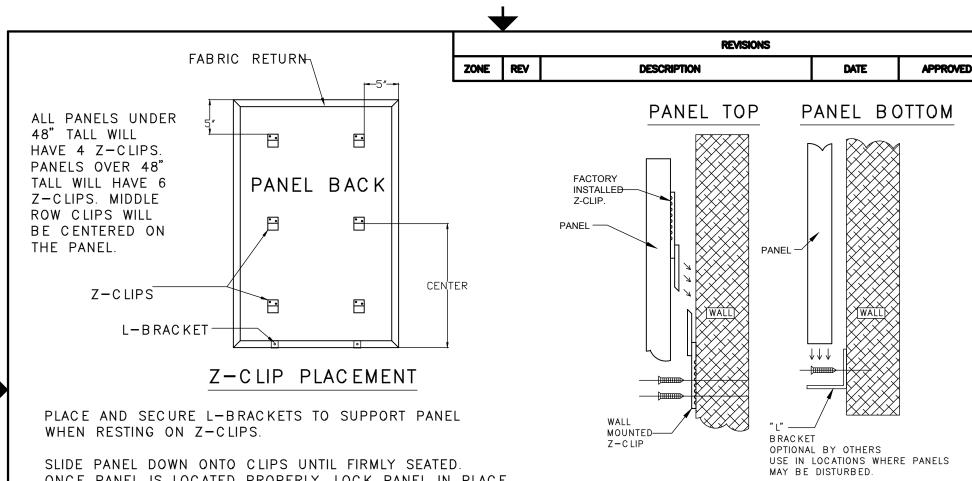
SLIDE PANEL DOWN ONTO CLIPS UNTIL FIRMLY SEATED.
